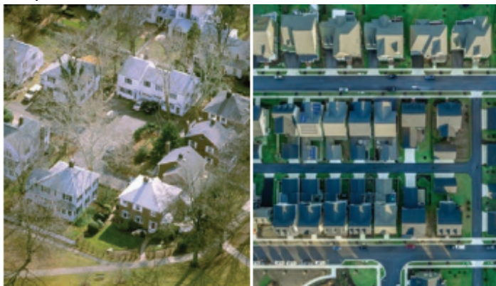
3 dwelling units/acre (left) and 14 dwelling units/acre (right). "Visualizing Density" by J. Campoli and A.S. MacLean.
