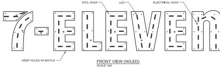
PRIMARY LEADS 1/2" CONDUIT-BLACK, WHITE, (100-240 VAC) AND GREEN (GROUND) (UL) APPROVED 100 WATTS 1/2" STR, CONNECTOR (UL APPROVED) TOP TBOTTOM : E L UL POWER SUPPLY ENCLOSURE W/ SWITCH-
