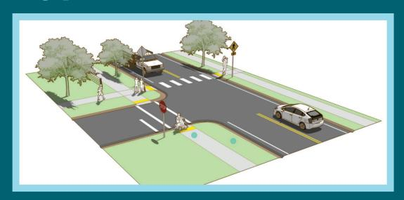
**Sidewalks** provide dedicated space intended for use by pedestrians that is safe, comfortable, and accessible to all. Sidewalks are physically separated from the roadway by a curb or unpaved buffer space.
