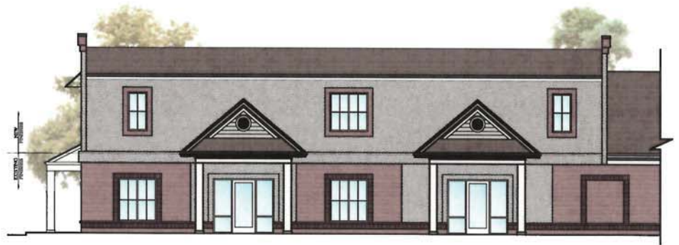
2 FRONT ELEVATION - PARKING LOT SIDE EL-1 3/16" = 1'-0"
