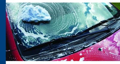
While you're at it, clean your wiper blades with a paper towel dipped in windshield washer fluid. This removes grime and oxidized rubber from the edge of the blade and helps prevent streaking. If streaks persist, you need new blade refills available from any auto parts store or discount chain.
