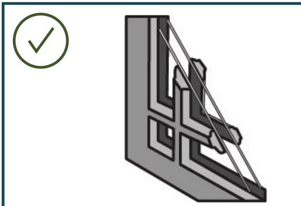
Appropriate simulated divided windows with muntins attached to both sides.
