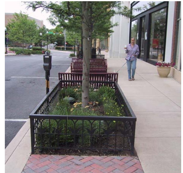
"Fence-style" tree guards are appropriate in areas with very high pedestrian traffic.
