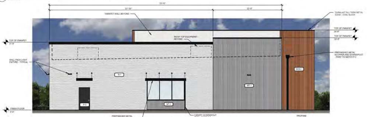
3 LEFT ELEVATION - FACING MYERS RD 3/16" x 1'-0"
