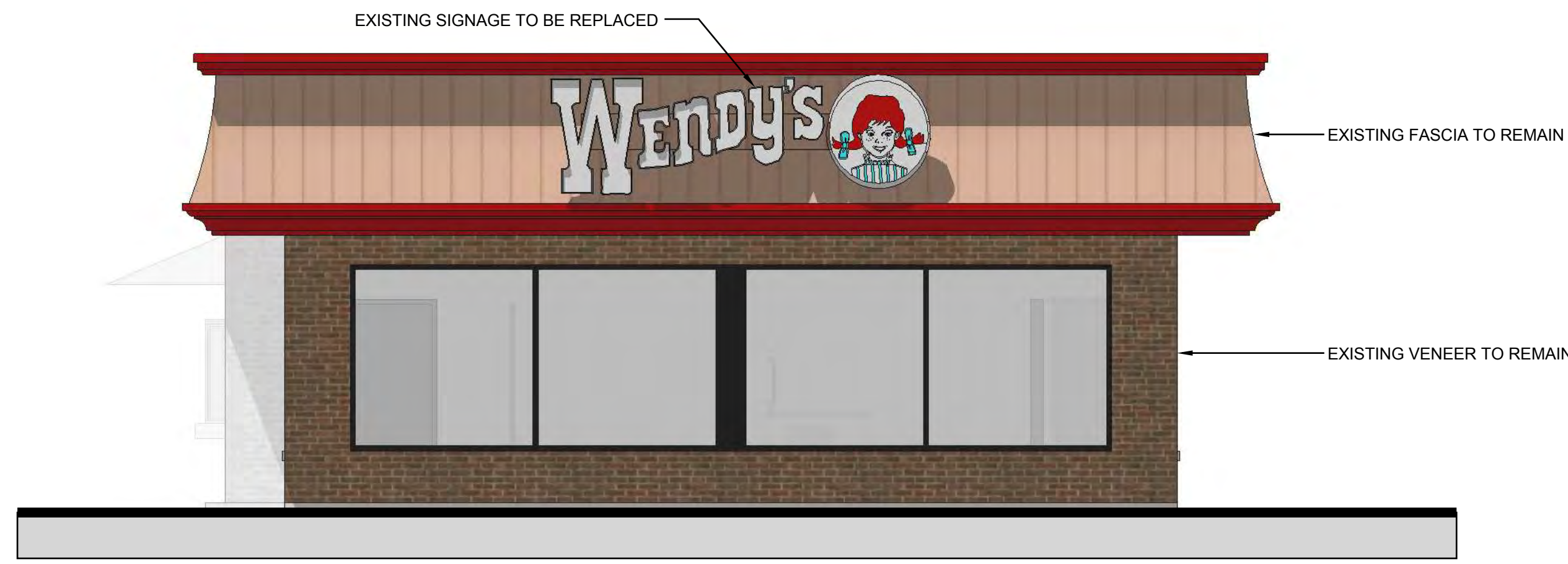
3 Existing Front Elevation 1/4" = 1'-0"
